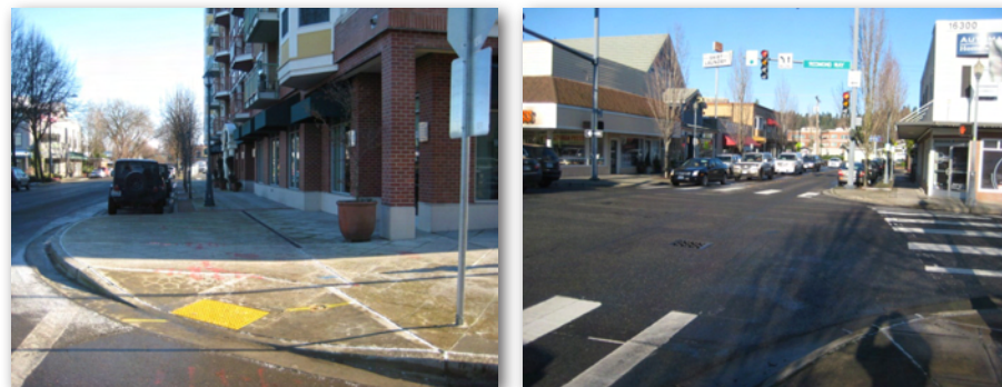
Curb extensions, well-marked crosswalks, wide sidewalks and Americans with Disabilities Act (ADA) compliant curb ramps help make Redmond streets safer and more accessible for all roadway users. Photos: Max Hepp-Buchanan
