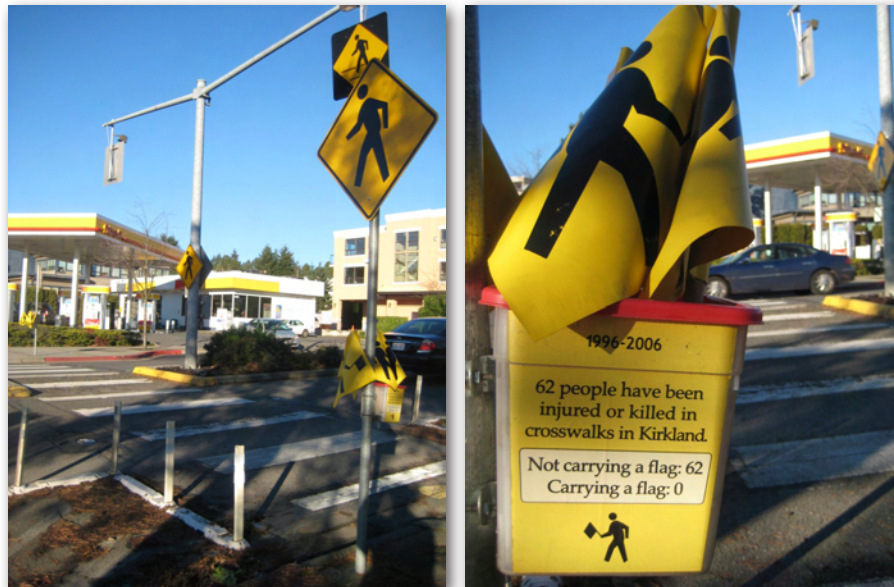
A crosswalk on one of Kirkland's busiest arterials uses buffers, curb extensions and a pedestrian refuge island for shorter crossing distances, as well as pedestrian crossing flags for increased visibility and safety. Photos: Max Hepp-Buchanan
